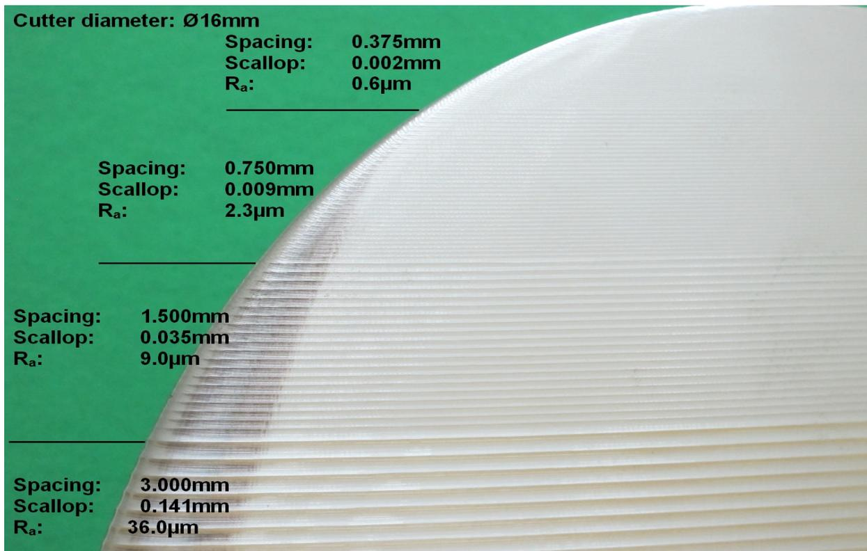
Figure 2: Finish machining with 16 mm cutter
