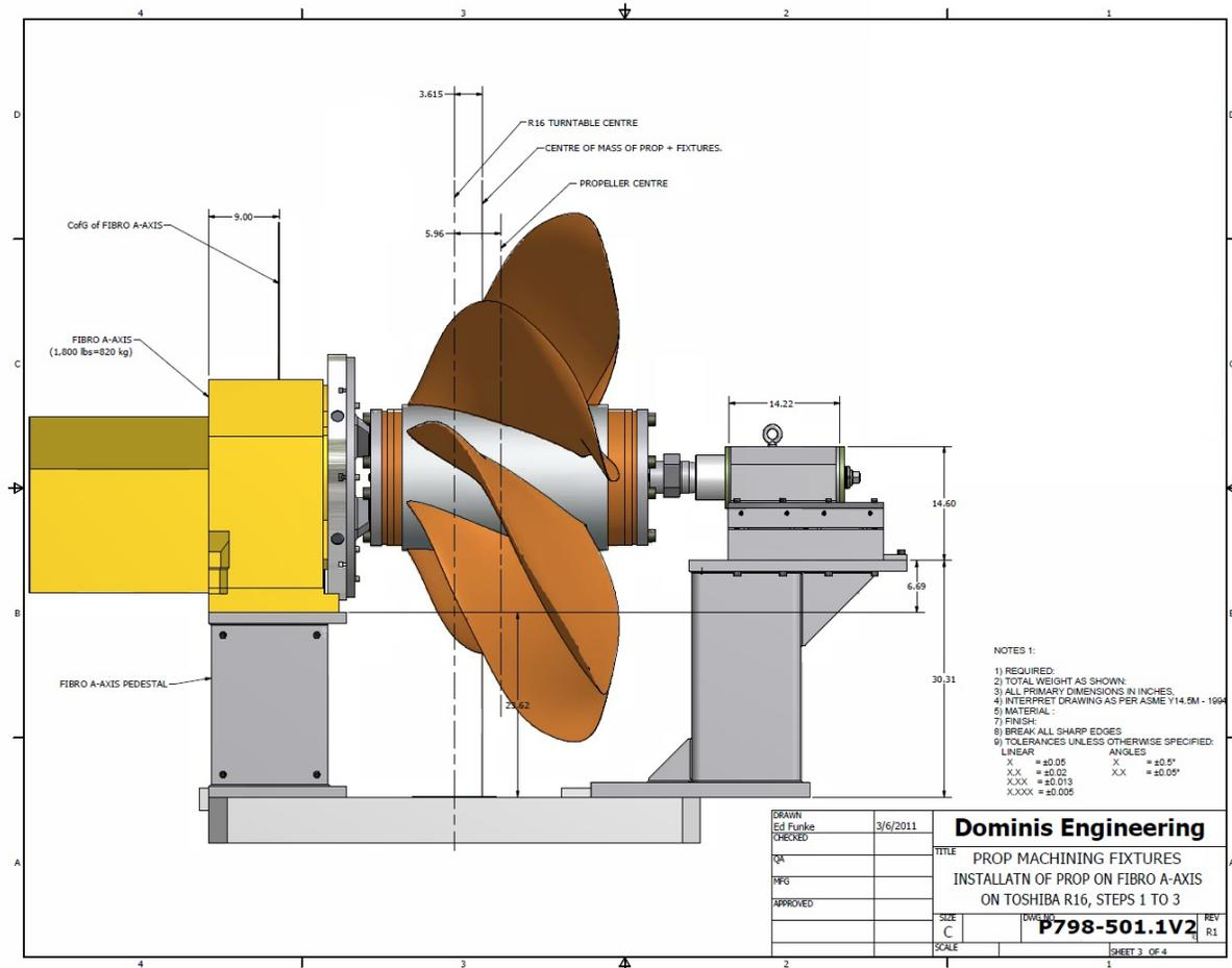
Figure 3: Set-up for 5-axis machining of monoblock propeller
