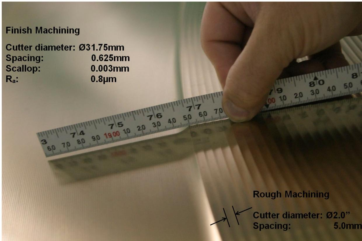
Figure 1: Finish machining with 1.25" ball nose cutter
