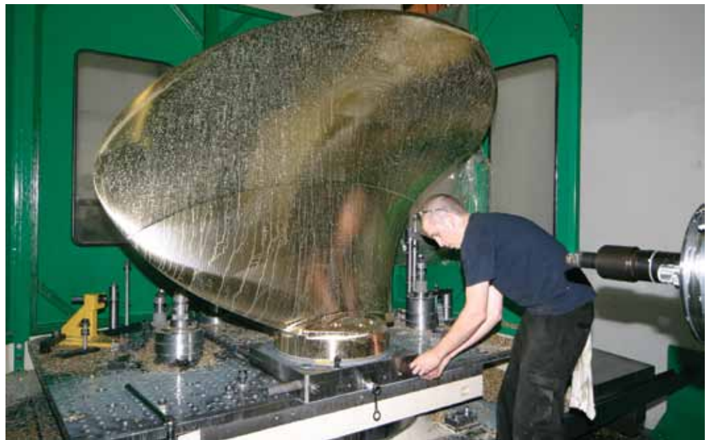
A Canadian Patrol propeller blade machined in Dominis Engineering's facility.
